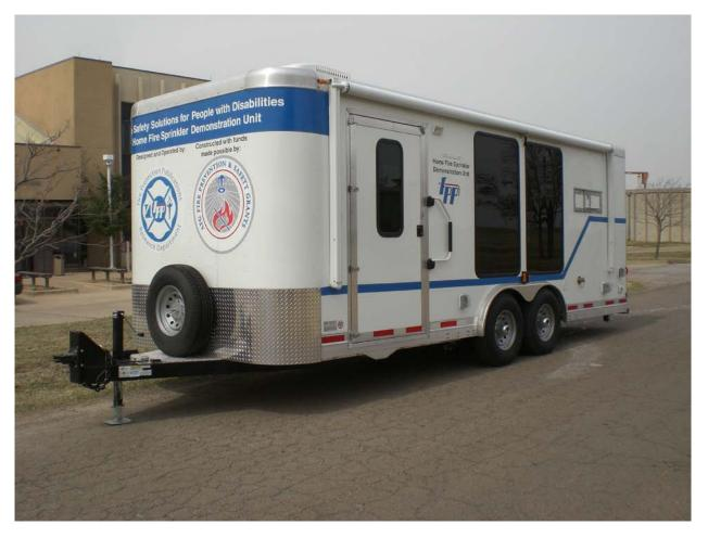
The design of the trailer consists of three rooms: An interior viewing room, a live fire demonstration (middle) room, and the sprinkler control room. The demonstrations may be viewed from the interior which is climate controlled, or externally from either side through large, low windows. The trailer has an ADA compliant ramp to bring people into the interior viewing room and a large retractable awning on the outside for shade when needed.
